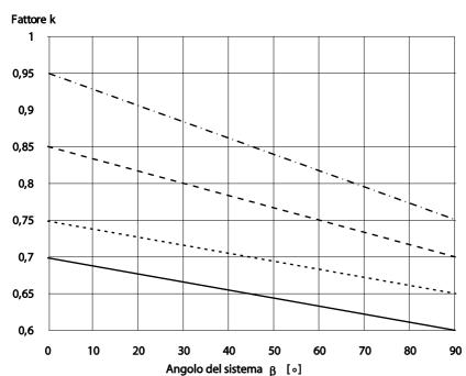
$0 < w \le 16.8$  $: A > 70 \text{ mm}^2$ Cu  $: A > 95 \text{ mm}^2$ Ac Al, Ad  $: A > 600 \text{ mm}^2$  $16.8 < w \le 28.5$  $19,6 \le A \le 70 \text{ mm}^2$ Cu :  $50 \le A \le 95 \text{ mm}^2$ Ac Al, Ad :  $300 \le A \le 600 \text{ mm}^2$  $28,5 \le w \le 42,8$ : A < 50 mm<sup>2</sup> Ac Al, Ad  $: 185 \le A < 300 \text{ mm}^2$ 42.8 < w: A < 185 mm<sup>2</sup> Al, Ad
