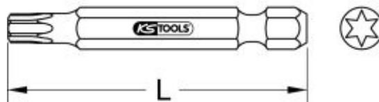
**BOITE DE 5 EMBOUTS DE VISSAGE TORX®, L.50 MM - 1/4" - T27**
