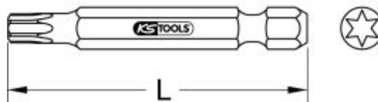
**BOITE DE 5 EMBOUTS DE VISSAGE TORX®, L.50 MM - 1/4" - T40**
