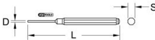
**CHASSE-GOUPILLE AVEC DOUILLE DE GUIDAGE Ø 3.4MM,
