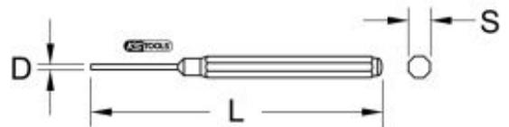
**CHASSE-GOUPILLE AVEC DOUILLE DE GUIDAGE Ø 4.9MM,
