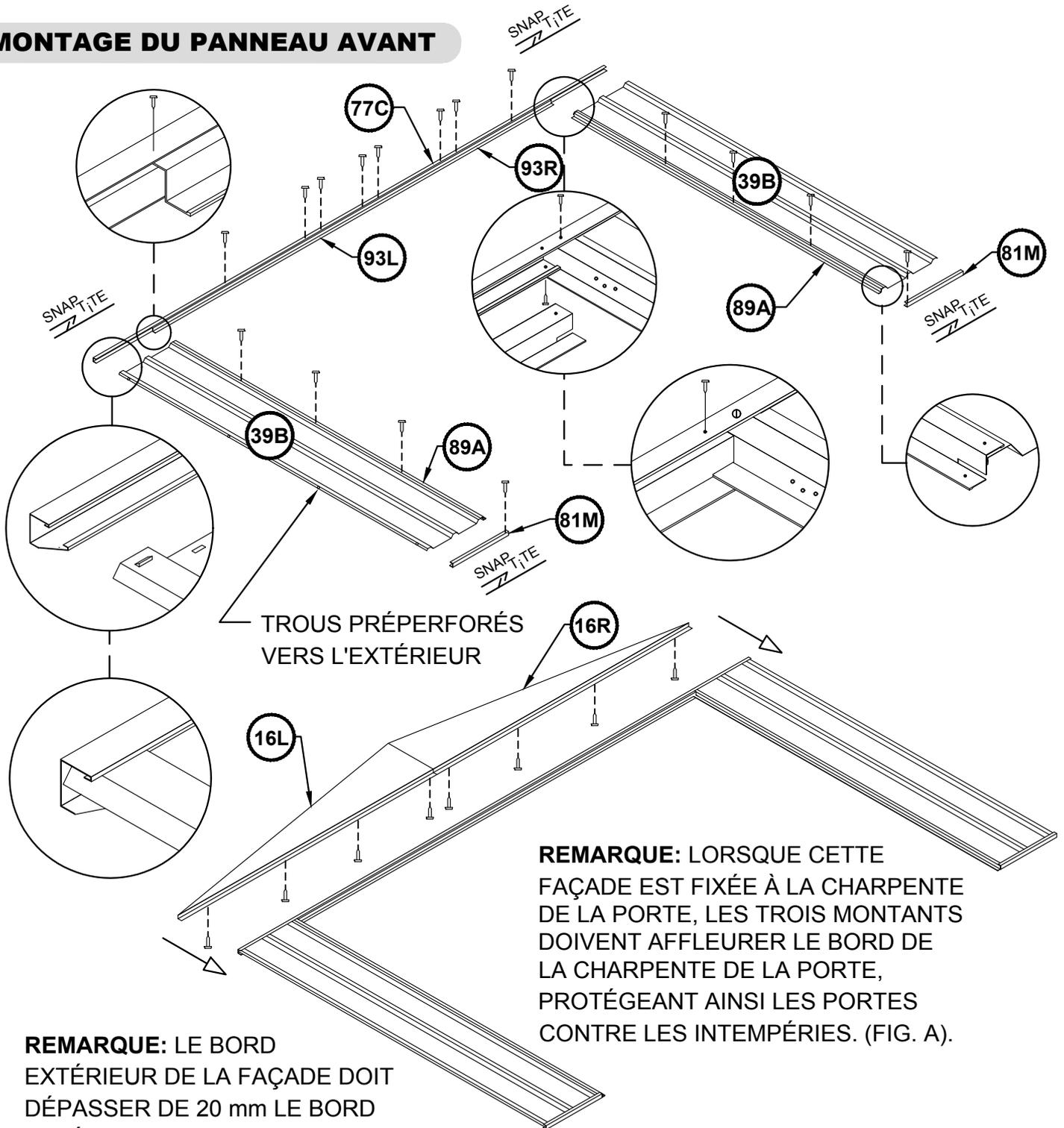
**REMARQUE:** LORSQUE CETTE FAÇADE EST FIXÉE À LA CHARPENTE DE LA PORTE, LES TROIS MONTANTS DOIVENT AFFLEURER LE BORD DE LA CHARPENTE DE LA PORTE, PROTÉGEANT AINSI LES PORTES CONTRE LES INTEMPÉRIES. (FIG. A).
