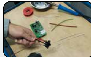
Pose de gaine thermo-rétractable Heat-shrink tubing installation
