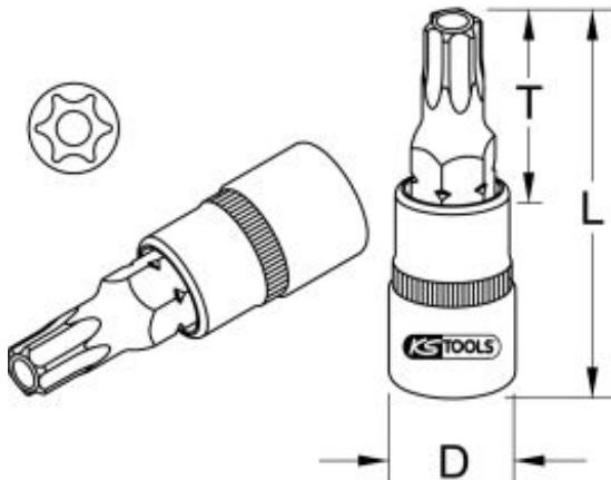
**DOUILLE TOURNEVIS ULTIMATE TORX® PERCÉ 3/8", L.50 MM - TB25**
