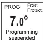
If you set a Frost Protection temperature (7°C), the programming is suspended.
