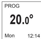
If the screen displays **PROG**, you are in a programming range in Comfort mode.
