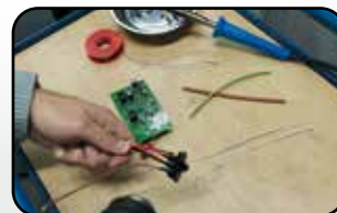
Pose de gaine thermo-rétractable Heat-shrink tubing installation
