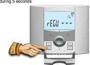
The display with the first parameter appears ( « rEGU »). - Once you entered in the menu, go to the parameter which you want change by using the keys (◄) or (►).
