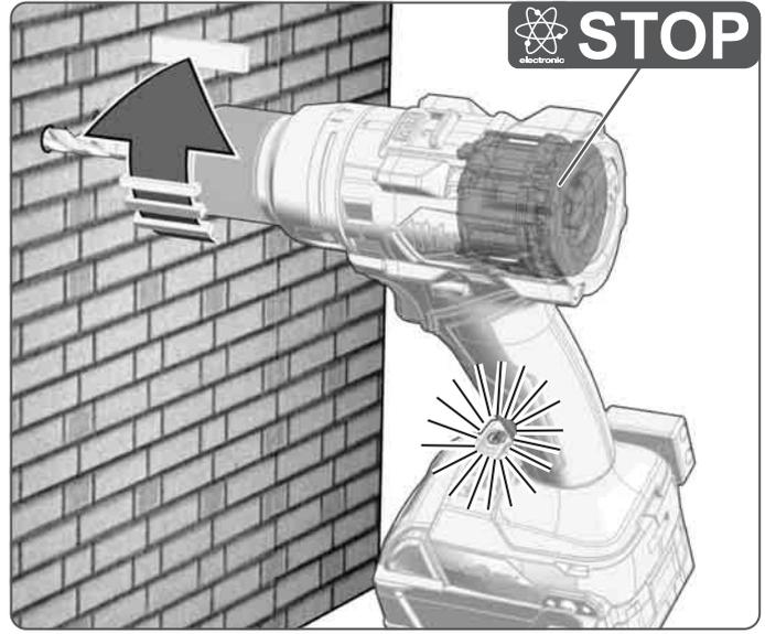
The machine has an overload and anti-kickback safety function and stops if it is overloaded.
