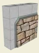
Clean Masonry Installation Scratch coat Setting bed  $Dutch\ Quality\ Stone^{\text{\tiny M}}$
