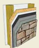
Wood Stud Installation Sheathing Weather resistant barrier Weather resistant barrier Metal lath Scratch coat Setting bed Dutch Quality  $Stone^{\text{TM}}$
