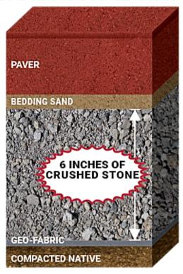
When laying different thickness of pavers or stones, adding a second layer 1/2" (13 mm) of loose bedding sand on top of the Gator Base™ is also an accepted method of installation.
