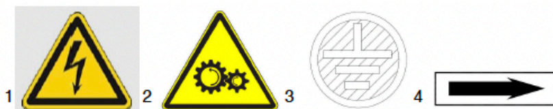
Fig. 1: Safety labels - 1 Warning of dangerous electrical voltage | 2 Caution rotating machine parts | 3 Grounding | 4 Direction of motor rotation
