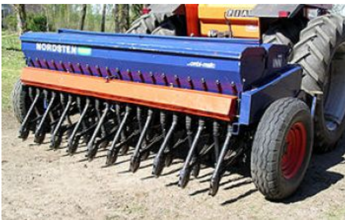
Sowing machine with seed drill concept
