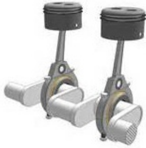
Piston-crank mechanism of an engine
