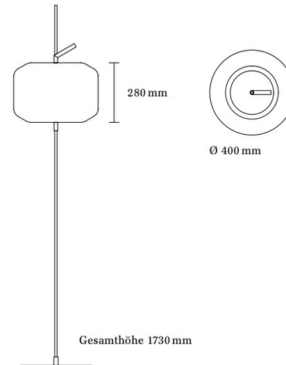
Material: weisses Polyethylen, Stahl matt vernickelt
