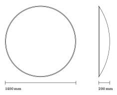
Membrane of fibre glass, steel frame
