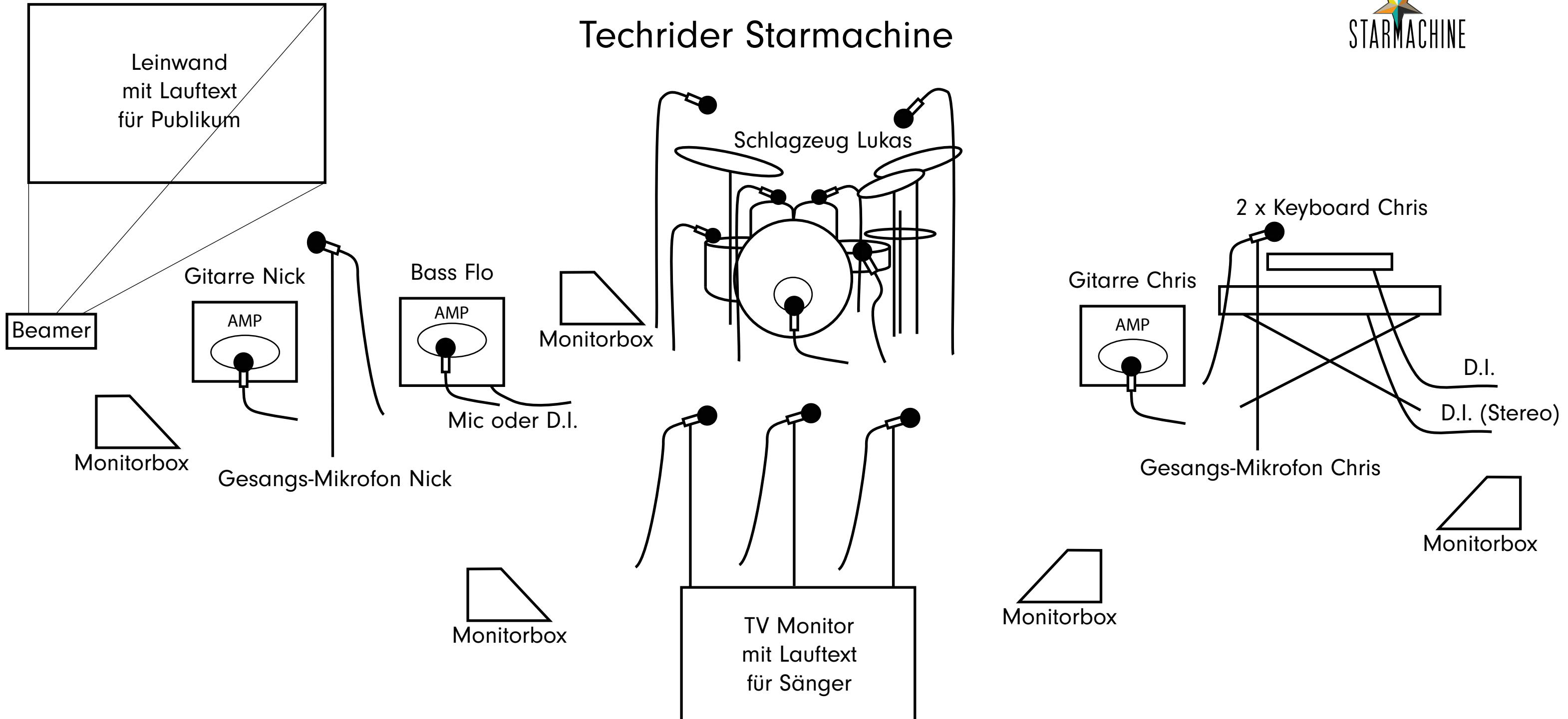
Mikrofonierung Drums: 1 x Bass, 1 x Snare, 3 x Toms, 2 Overhead (incl XLR)
