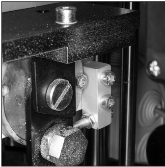
Hand lever adjusting screw. (front to back)
