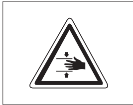
Risk of crushing
