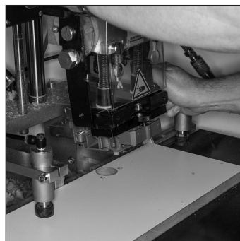
Press hand lever downwards.
