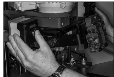
Press the Start buttons (the motor bracket moves downwards)
