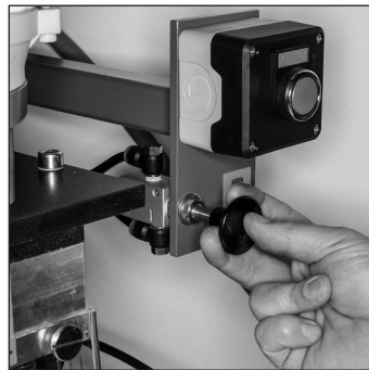
Clamp the hold-down devices.
