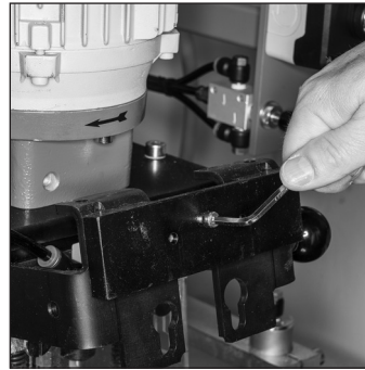
Side-to-side adjustment on ID arm plate.
