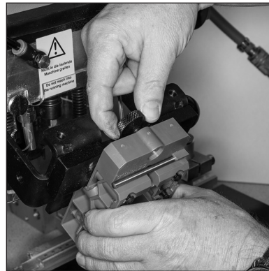
Fix ID in place by tightening clamp screw
