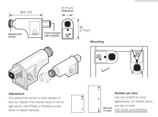
**Important:** Use a 65° angle for best mounting results. Pilot drill 2.3 mm [Ø3/32"] and 1/4" deep for a #6 x 3/4" Pan head screw recommended. Mount in upper corner on hinge side.
