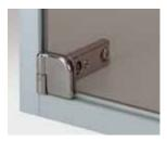
Stick the double-sided adhesive pad on the corner of the glass door. Peel off the protective foil. Place the glass door, the side with the pad facing outwards, into the already mounted hinge. Tighten the fixing screw.
