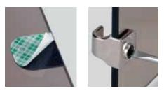
Decidethe pull position, stick the double-sided adhesive pad onto the glass door. Peel off the protective foil. Place the glass door, the side with the pad facing outwards, into the pull. Tighten the fixing screw. (max. 2 Nm).
