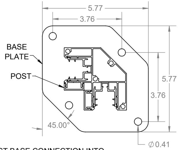
POST BASE CONNECTION INTO WOOD WITH THROUGH BOLTS
