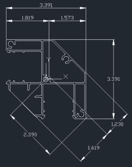
Section Modulus-based on principal Moment of Inertia:  $Sx = Ix/Cx = 0.724/(1.619) = 0.447 \text{ in}^3$  $Sy = Iy/Cy = 1.954/(2.39) = 0.818 \text{ in}^3$
