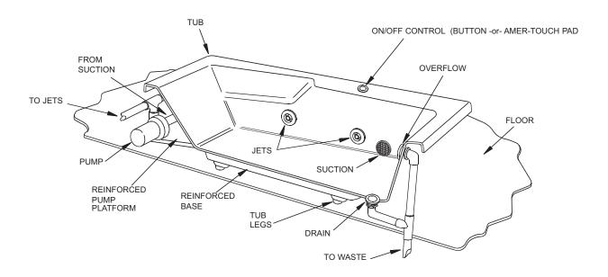
SUCTION FITTING: Feeds water to the pump. The suction fitting should be kept clean and free of debris. DO NOT RUNTHE PUMP IF THE SUCTION COVER IS NOT IN PLACE.
