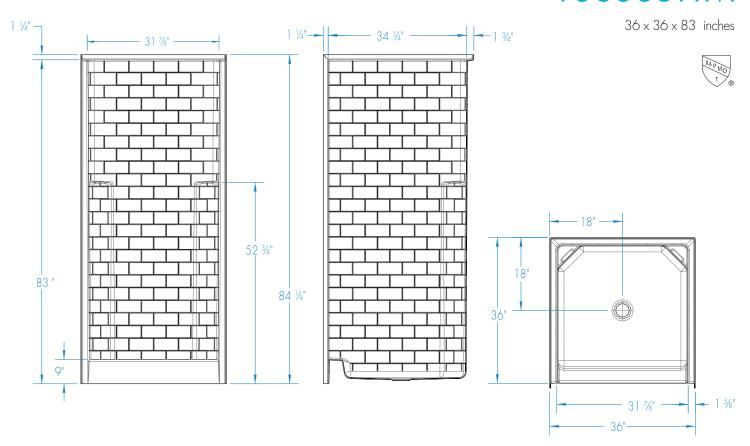
$\label{eq:FEATURES} \textbf{ Dimensional Tolerance} \pm \textbf{\%}''. \textbf{ Dimensions needed for site preparation should be measured from the unit. Aquatic assumes no responsibility for preparatory work.}$
