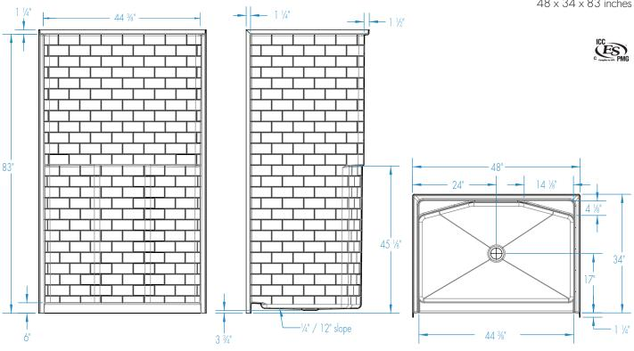
$\label{eq:FEATURES} \textbf{ Dimensional Tolerance} \pm \textbf{\%}''. \textbf{ Dimensions needed for site preparation should be measured from the unit. Aquatic assumes no responsibility for preparatory work.}$
