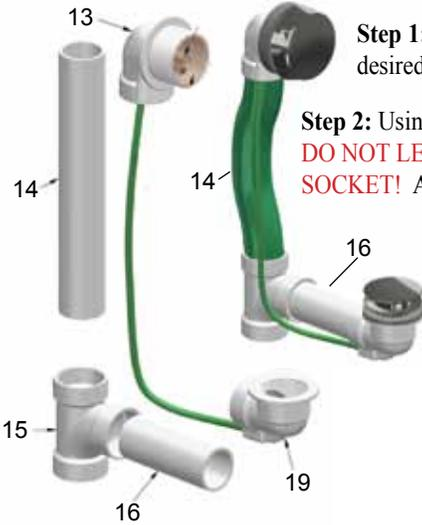
**Step 1:** Cut the 1½” Schedule 40 (or Flexible PVC) overflow pipe and drain pipe (*Items 14 and 16*) to the desired lengths to fit the tub.
