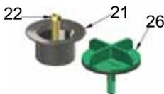
**Step 7:** Screw the strainer test plug (*Item 26*) into the strainer body (*Item 21*) and test the system (*Figure 5*).
