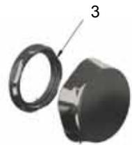
**Step 5:** Screw on the overflow elbow (OE) nut (*Item 3*) from inside of the tub (*Figure 2*). **HAND TIGHTEN ONLY** until the nut is snug and the gasket is only slightly compressed against the back of the tub. **You must get a minimum of 1½ turns when installing the nut.** If there are not enough threads sticking through the tub to get the nut installed, remove the thick gasket (*Item 12*) and replace it with the thin gasket (*Item 11*).
