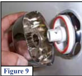
Secure the faceplate (*Item 2*) to the faceplate adapter (Figure 9) using either the faceplate screw (*Item 1*) (Figure 10). (Leave the plastic sleeve on threads to help align the screw.)
