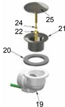
**Step 6:** Secure the drain elbow (*Item 19*) and drain flange gasket (*Item 20*) under the tub by screwing in the strainer body (*Item 21*) through the tub drain hole from inside the tub (*Figures 3 and 4*). If desired, a putty or sealant may be used between the flange of the strainer body and the tub. **CAUTION: Do not use linseed oil based putty products. Use only thread compounds specifically intended either for ABS or PVC assembly.**
