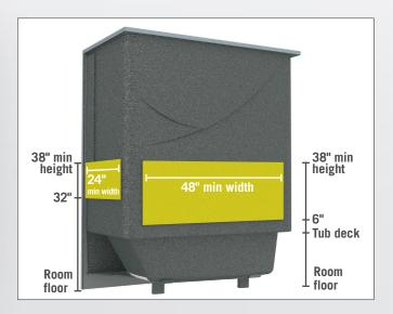
**Minimum reinforced areas for a bathtub:** Reinforced area on the <u>back wall</u> should start at least 6" above the tub deck and extend to a minimum height of 38" from room floor, with a minimum width of 48". Reinforced area on the <u>side walls</u> should start at least 32" from room floor and extend to a minimum height of 38", with a minimum width of 24".<sup>3</sup>
