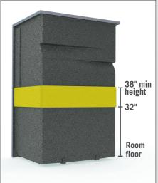
Minimum reinforced areas for a shower: Reinforced area on <u>all</u> walls should start at least 32" from room floor and extend to a minimum height of 38".
