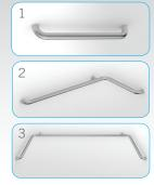
AKER's Outlook *plus* textured stainless steel grab bars feature an easy to clean smooth surface. Straight $^1$ , L-shaped $^2$  or U-shaped $^3$ , in multiple dimensions, there is one for every need. All grab bars are 1  $^1$ 4" in diameter, securely bolted through the wall, and are designed and tested to withstand up to **300** lb of pressure as per major accessibility building codes.
