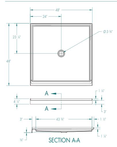
FEATURES Dimensional Tolerance ± 36". Dimensions needed for site preparation should be measured from the unit. Manufacturer assumes no responsibility for preparatory work.
