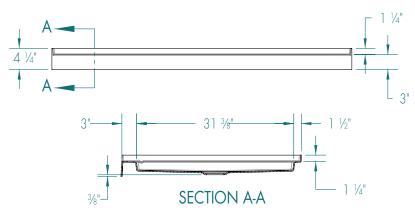
$\textbf{FEATURES} \qquad \text{Dimensional Tolerance} \pm \textbf{\%}''. \text{Dimensions needed for site preparation should be measured from the unit. Manufacturer assumes no responsibility for preparatory work. } \\$
