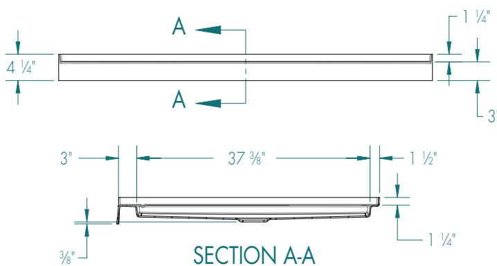
**FEATURES** Dimensional Tolerance  $\pm \frac{3}{16}$ ". Dimensions needed for site preparation should be measured from the unit. Manufacturer assumes no responsibility for preparatory work.
