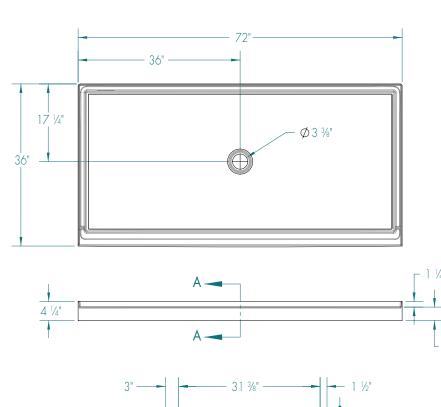
FEATURES Dimensional Tolerance ± 36". Dimensions needed for site preparation should be measured from the unit. Manufacturer assumes no responsibility for preparatory work.
