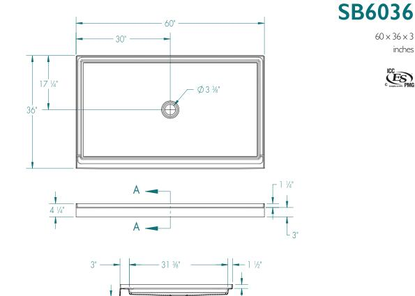
FEATURES Dimensional Tolerance ± 36". Dimensions needed for site preparation should be measured from the unit. Manufacturer assumes no responsibility for preparatory work.
