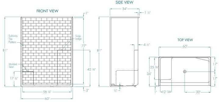
FEATURES Ibs Dimensional Tolerance ± 36". Dimensions needed for site preparation should be measured from the unit. Manufacturer assumes no responsibility for preparatory work.
