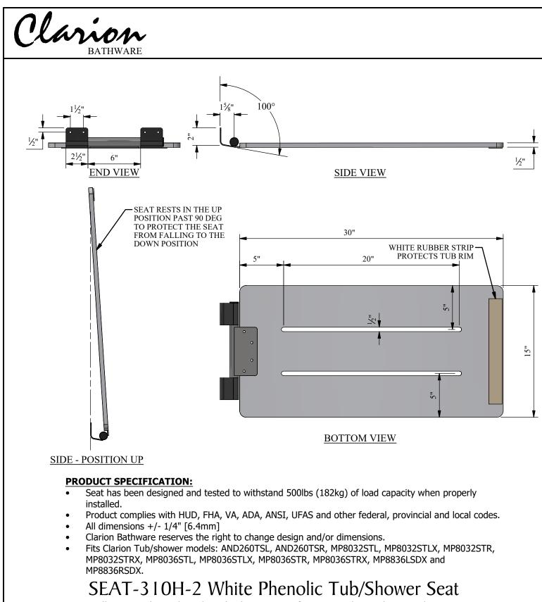
Wall Mounted Bench-Style Tub/Shower Transfer Seat With Stainless-Steel Hinges
