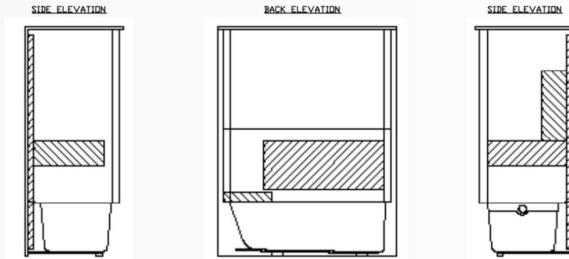
← **Standard MS Core Structural Reinforcement Layout**
