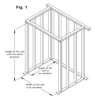
At this point of the installation, the method used depends upon whether or not there will be access to the back and sides of the unit after it is installed to allow installation of the dome. If there will be access to the back and sides of the unit after installing the unit, METHOD 1 should be used to install a unit with a cap. If there will not be access to the unit after it is installed, METHOD 2 should be used to install the unit.
