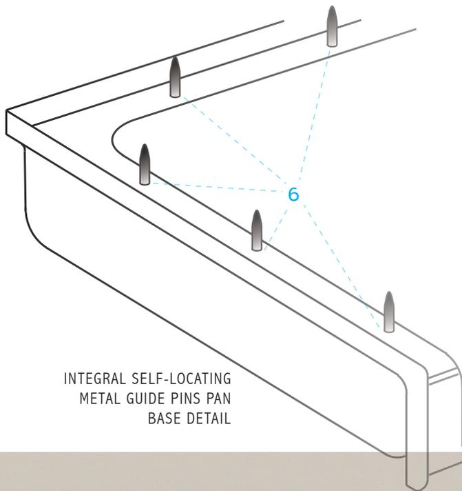
INTEGRAL SELF-LOCATING METAL GUIDE PINS PAN BASE DETAIL
