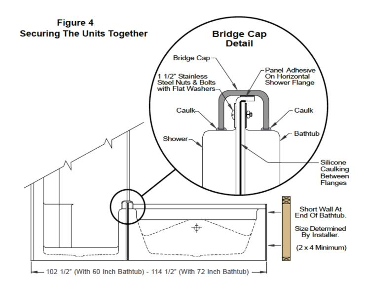
**NOTE:** The front facing flange and the horizontal facing flanges on the tub and the shower should align within 1/4".
