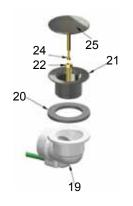
Step 10: Rotate the faceplate CLOCKWISE to the fully-closed position. Install the core guide (*Item 22*) into the strainer body using a screwdriver or 7/16" socket (Figure 11). (See core guide instruction card included with kit.) The core guide should be screwed in until it is snug against the bottom of the drain elbow. Insert the stopper (*Item 24*) into the core guide (*Item 22*) (Figure 12).
