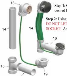
Step 1: Cut the 1½" Schedule 40 (or Flexible PVC) overflow pipe and drain pipe (*Items 14 and 16*) to the desired lengths to fit the tub.
