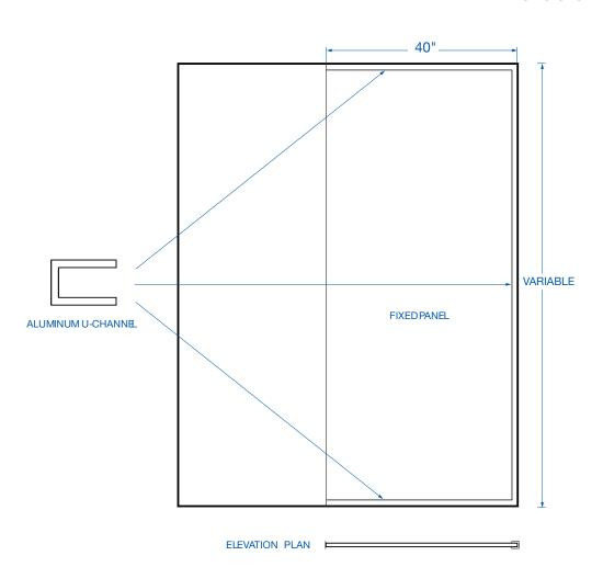
\*NOTE: These measurements are based on a standard 40" x 96" enclosure. Heights and Widths are variable and can be ordered to fit specific project requirements.
