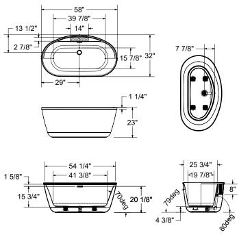
(a) Recommended faucet area 1 section of 14" (L) x 2 7/8" (W). Depth recommended for straight pipes 8".
