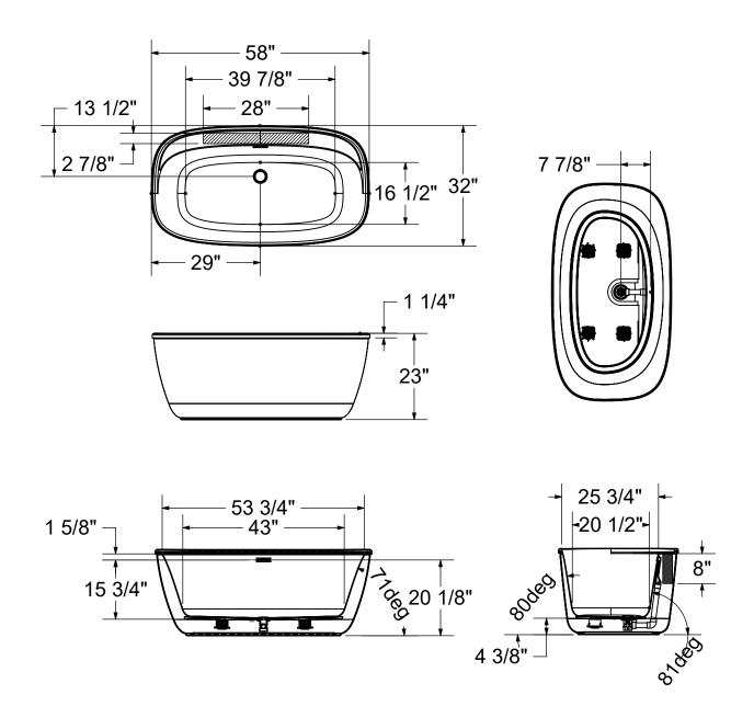
(:) Recommended faucet area 1 section of 28" (L) x 2 7/8" (W). Depth recommended for straight pipes 8".
