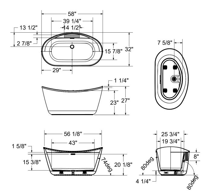
(:) Recommended faucet area 1 section of 14 1/2" (L) x 2 7/8" (W). Depth recommended for straight pipes 8".
