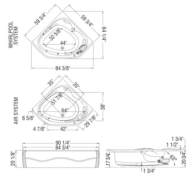
( ): Indicates Whirlpool jets positioning( ): Indicates airjets positioning
