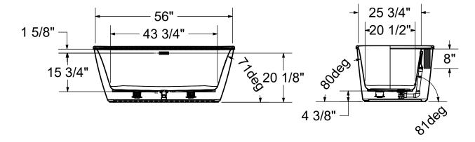
(: Recommended faucet area 1 section of 45" (L) x 2 7/8" (W). Depth recommended for straight pipes 8".
