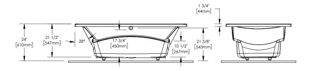
Wood support design may vary. All dimensions are approximate. Structure measurements must be verified against the unit to ensure proper fit.
