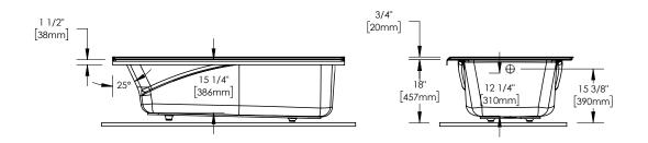
Wood support design may vary. All dimensions are approximate. Structure measurements must be verified against the unit to ensure proper fit.
