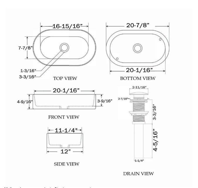
All dimensions are approximate. Structure measurements must be verified against the unit to ensure proper fit.
