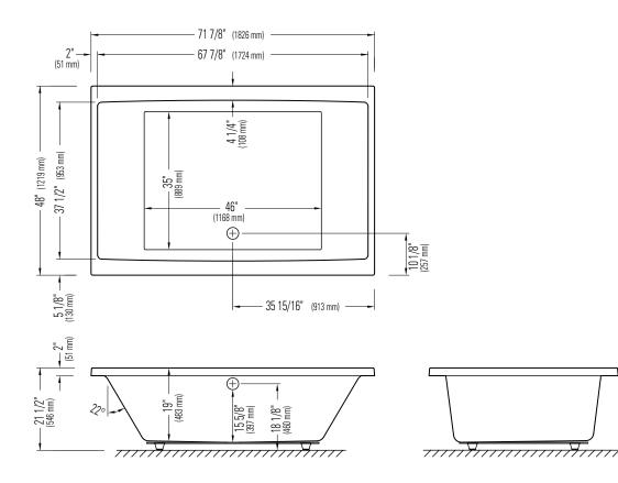
\*A bathtub fitted with back jets can cause the pump to protrude by approximately 3 $^{\prime\prime}$  from the overall dimension.
