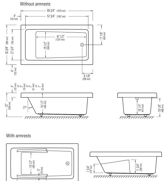
\*A bathtub fitted with back jets can cause the pump to protrude by approximately 3" from the overall dimension.
